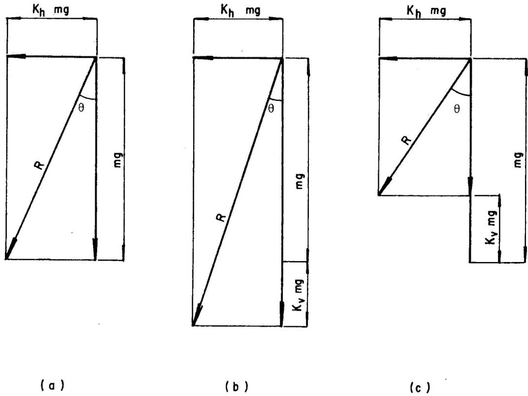
FIG. 7 SEISMIC COEFFICIENTS AND FORCES
