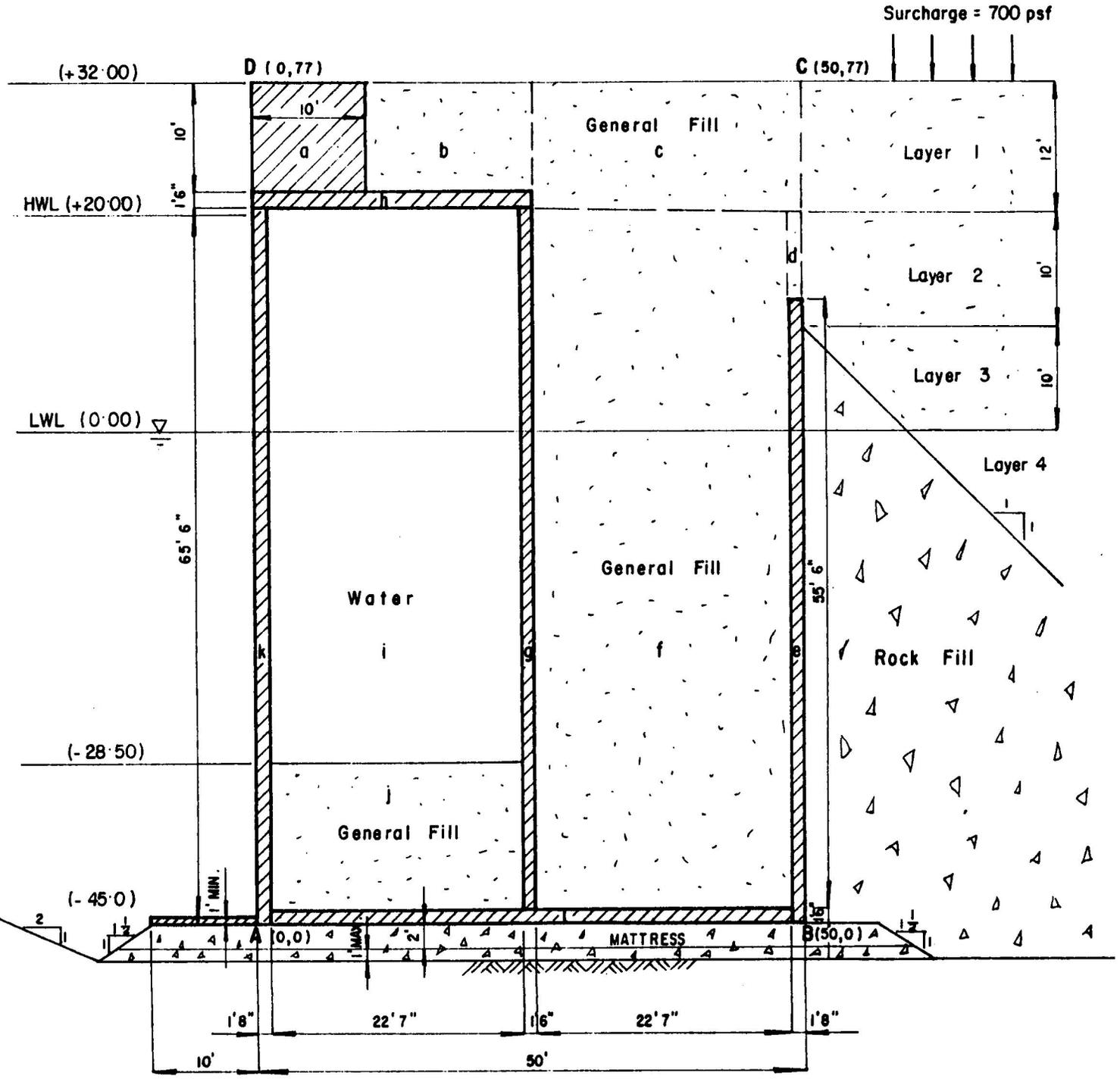
FIG. 1 ASSUMED CROSS SECTION OF MARGINAL WHARF RETAINING WALL AND BACKFILL
