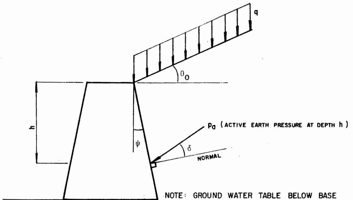
FIG. 9 DYNAMIC ACTIVE EARTH PRESSURE AT DEPTH  $h$  DUE TO SURCHARGE
