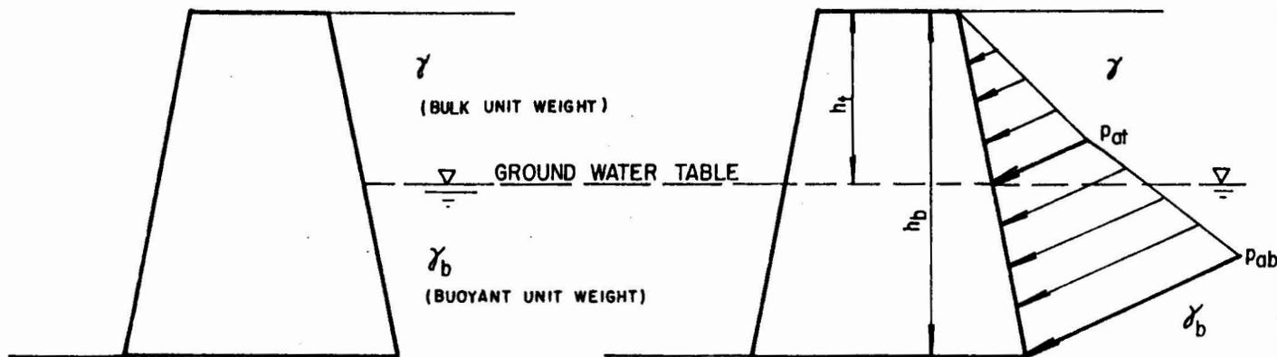
FIG. 11 DYNAMIC ACTIVE EARTH PRESSURES WITH GROUND WATER TABLE
