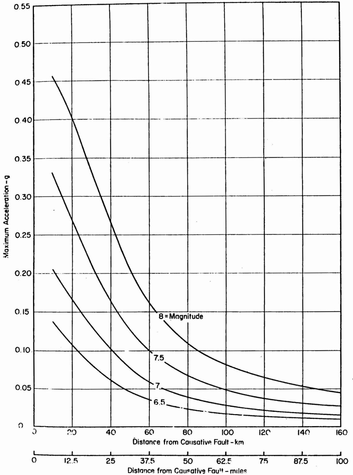
FIG. 4 VARIATION OF MAXIMUM ACCELERATION WITH EARTHQUAKE MAGNITUDE AND DISTANCE FROM CAUSATIVE FAULT
