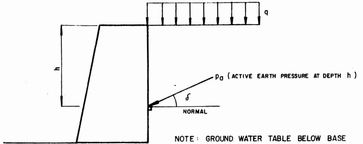
FIG. 10 DYNAMIC ACTIVE EARTH PRESSURE AT DEPTH  $h$  ON A VERTICAL WALL
