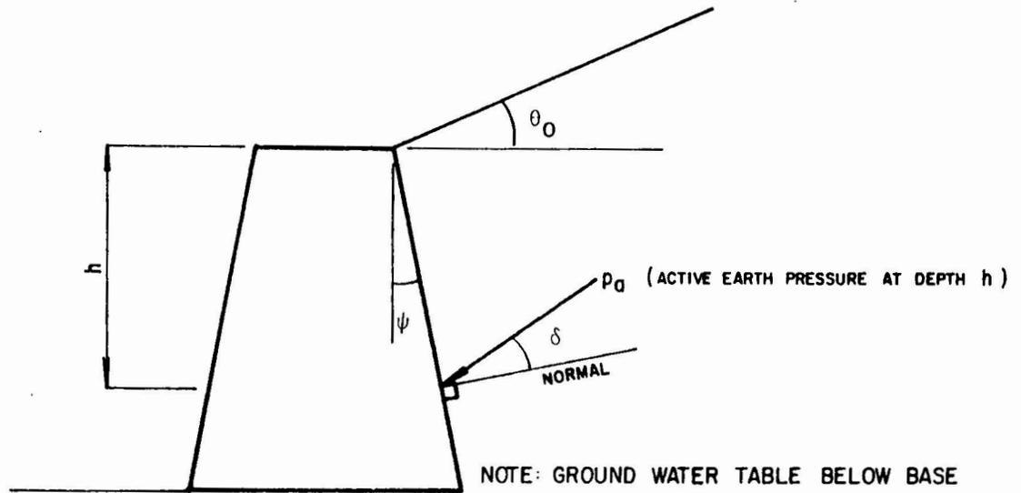
FIG. 8 DYNAMIC ACTIVE EARTH PRESSURE AT DEPTH  $h$  FOR A SLOPING BACKFILL
