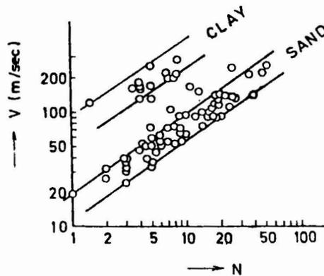
FIG. 6 SHEAR WAVE VELOCITY AND N-VALUE OF STANDARD PENETRATION TEST
